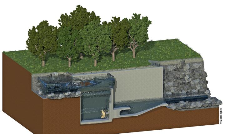
Global Hydro developed the Kaplan EVO to be a fully submersible Kaplan turbine for use in the shaft power plant.
